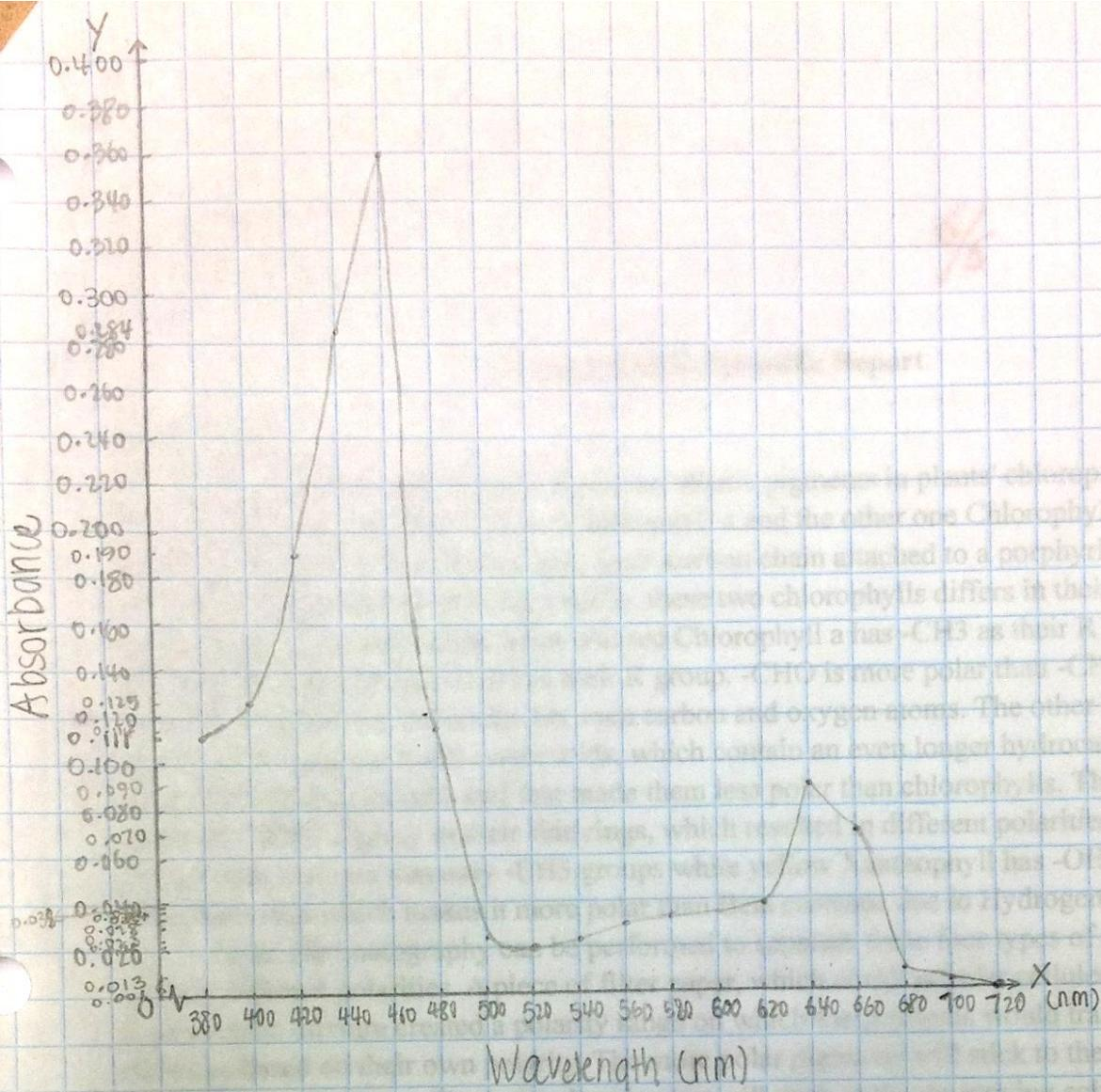
Figure 2. The Absorbance of Chlorophyll b Corresponding to Wavelength 380-720 nm
